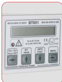
Controlhousing in accordance with ATEX
