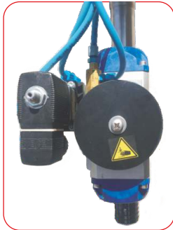
Automatic protection device, interlocking
